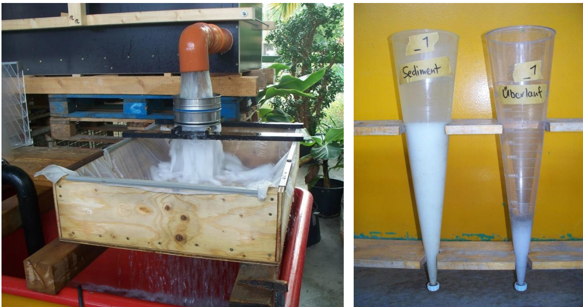
Figure 8: Left: Overflow fabric sieve for recovery of model sediment (the round coarser sieves above acted as antispash protection only). Right: Imhoff cones for determination of sediment volume after 24 h of settling
